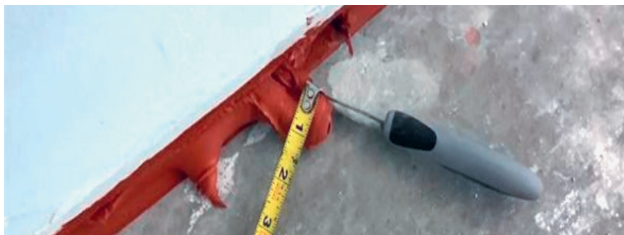
Fig.9: Sealant thickness measurement when wet
